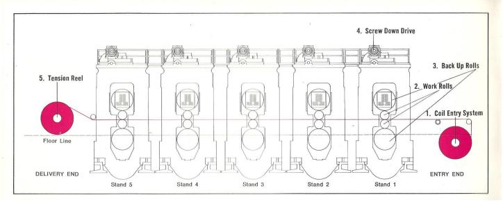
Then the steel was annealed to soften it and make it workable. The annealed steel then went through the 'temper mill' where two pairs of work rolls provided the specified hardness and
